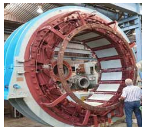
Fully Reconditioned Stator at Marthinusen & Coutts
