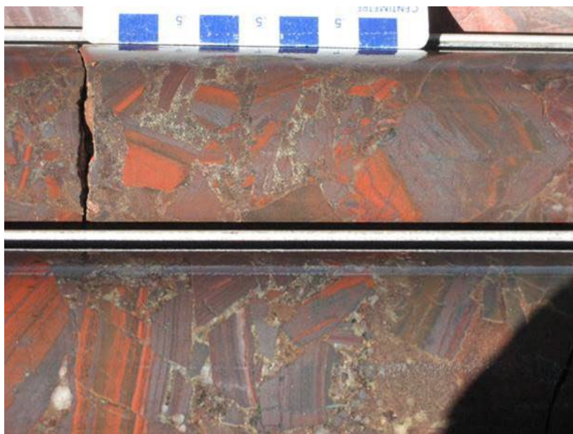
Figure 19: Hematite-rich jaspilitic BIF from MPD001 below 1,288m
