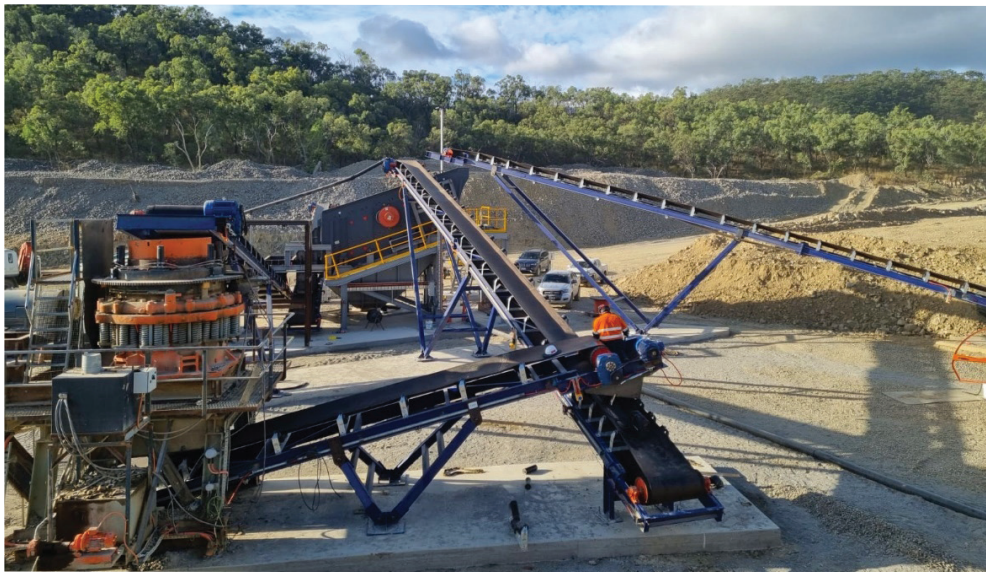
Newly installed screening and crushing plant.
